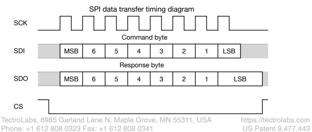
When an SPI data transfer is in initiated, the master device sends an 8-bit command to the MicroRNG device while the MicroRNG sends an 8-bit response (for the previous command) to the master device. The master device, therefore, will need two transfers to send a command and receive its response value.
